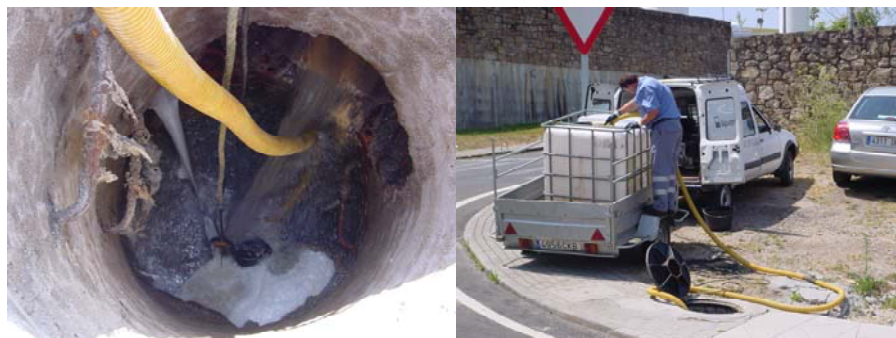
Figure 6-3. Collection and transport of hospital wastewater to feed the pilot plant.
