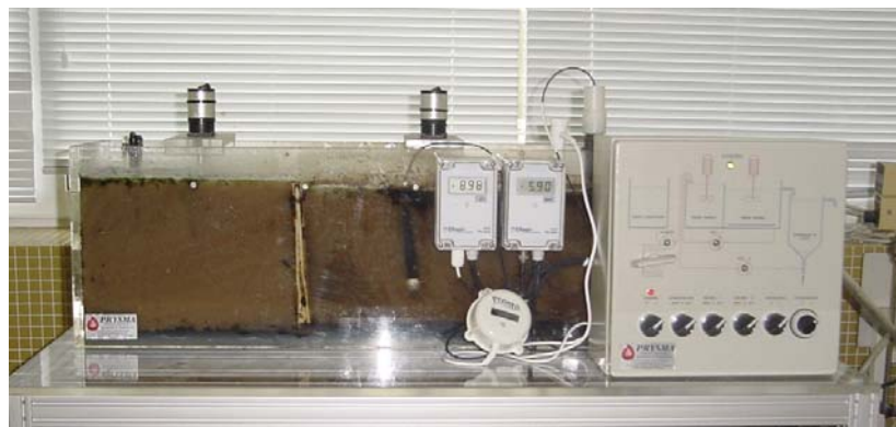
Figure 4-1. Activated sludge pilot plant.
