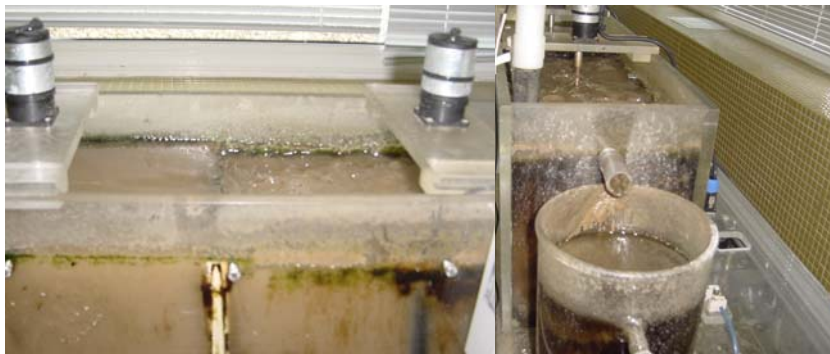
Figure 4-3. Details of the activated sludge pilot plant.
