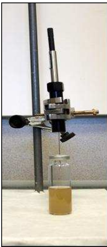
Figure 2-3. Set-up used in the Solid Phase Micro-Extraction (SPME) step for the determination of the total load of musk fragrances
