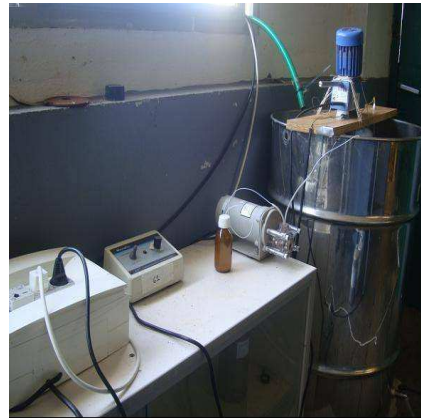
Figure 5-2. Picture showing the primary settler (left) and the mixing tank (right) with the spiking pump and PPCPs solution
