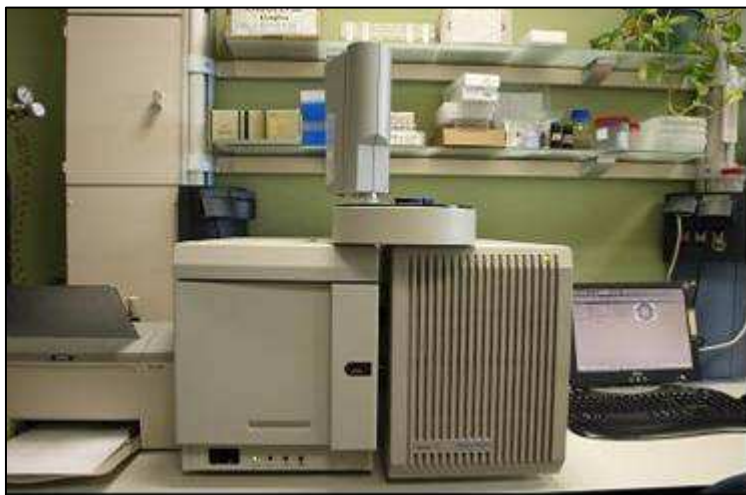
Figure 2-4. Varian Saturn 2100T GC/MS/MS used for the determination of anti-inflammatories, musk fragrances, carbamazepine and diazepam.
