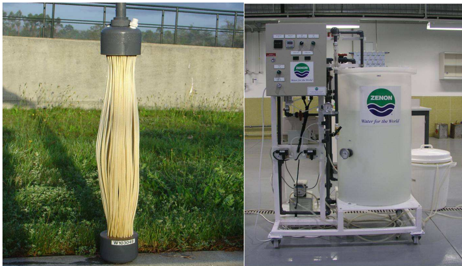
Figure 4-1. Membrane Module ZeeWeed-10 and Bioreactor
