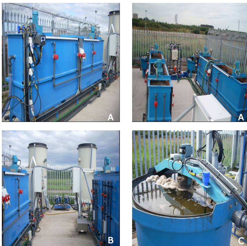
Figure 3-2. Pilot-scale plant consisting of aeration tanks (A), primary settlers (B) and secondary settler (C)
