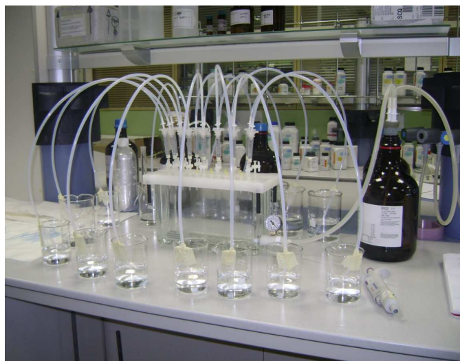
Figure 2-2. Manifold used in the Solid Phase Extraction (SPE) step for simultaneous concentration of different samples
