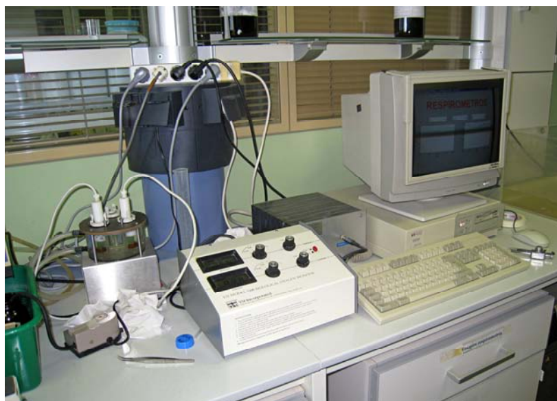
Figure 3.2. Respirometry system: left, thermostatic test cells; centre, biological oxygen monitor; right, data acquisition system.
