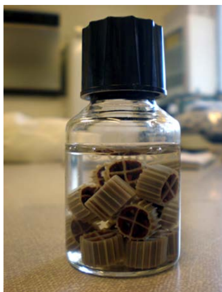
Figure 6.2. Vessel prepared to perform a SAA test with Kaldnes K1 rings (picture by Sandra Martínez and Zaira Hernando).
