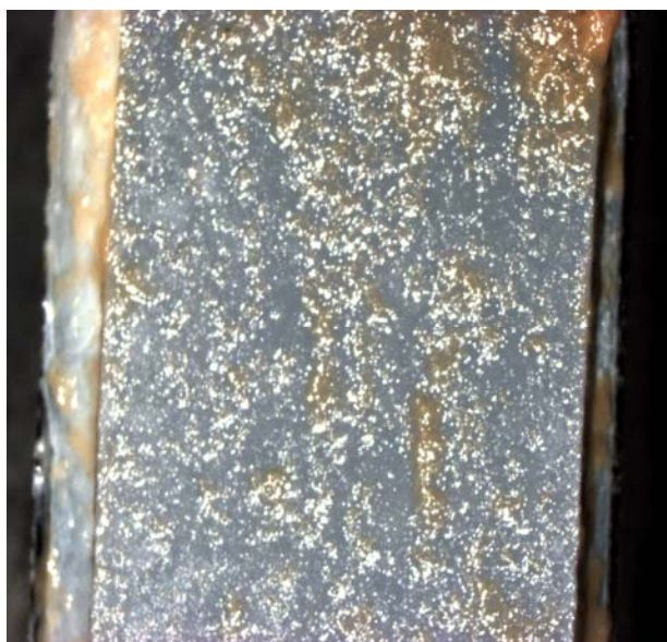
Figure 7.6. Sample of biofilm on the PVC surface of a removable sample collector, 6.5x, day 7 of test 4 (with NaCl).
