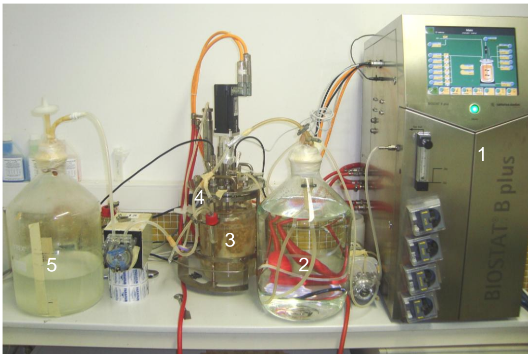
Figure 5-21. Stirred tank reactor (STR) configuration with P. chrysosporium immobilized in polyurethane foam and a continuous air flow. Symbols: (1) module operator service program, (2) feed medium port, (3) reactor vessel filled with immobilized fungus, (4) effluent sampling, (5) effluent reservoir.
