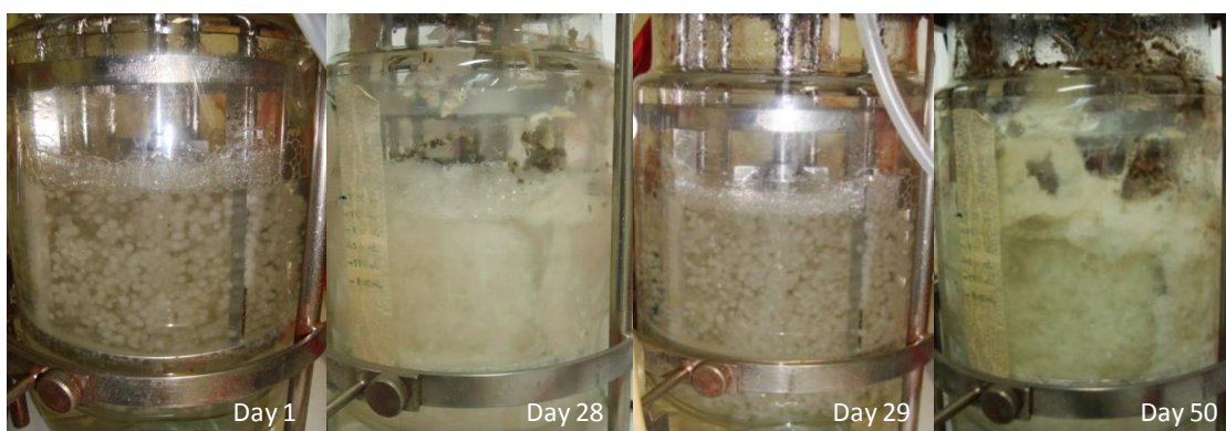
Figure 4-29. Appearance of the STR during the continuous experiment
