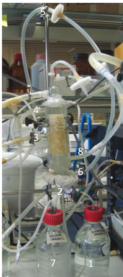
Figure 5-3. Fixed-bed reactor configuration with P. chrysosporium immobilized in polyurethane foam and a continuous air flow. Symbols: (1) feed medium reservoir, (2) feed addition port, (3) middle port, (4) upper port, (5) air supply, (6) air supply port, (7) effluent reservoir, (8) thermostated water.
